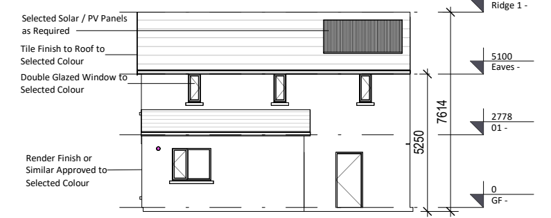
④ Rear Elevation End Terrace- 1 : 200
